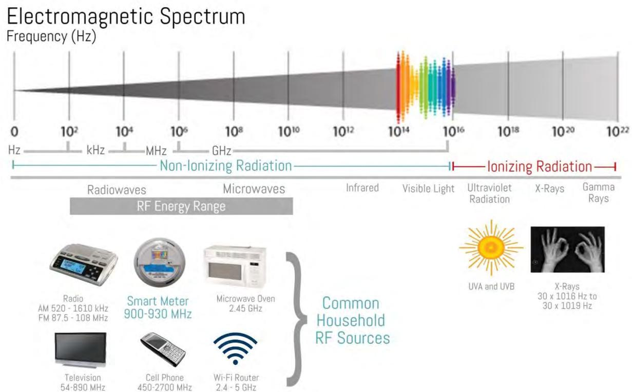
Figure 1. Electromagnetic Spectrum and RF Sources
